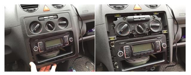
Remove plastic trim around the radio and heating/ac control panel. Locate torx screws fastening the radio and a/c panel, loose them to remove both parts.
