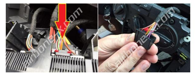
Remove connector from the climate control panel. Work on to remove insulation tape from the harness to get access to two mentioned wires as shown bellow.
