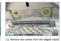
11. Remove the tripod of the tailgate trim board, there're two screws, remove them
